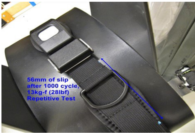
Figure 2. Failed test where to pass the standard a maximum of 10mm slip is permitted
