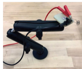
Figure 1. A surrogate cigarette flammability test apparatus
