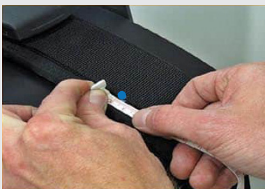
Figure 2. At the end of the test the blue dots are still within 10mm of each other: PASS
