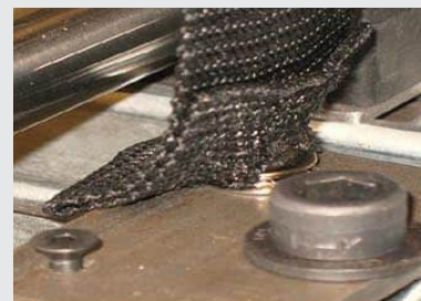
Figure 4. Grommet fixture undergoing a static load test: FAIL
