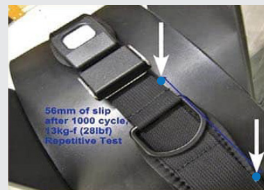
Figure 3. At the end of the test the blue dots are more than 10mm (i.e. 56mm) apart: FAIL
