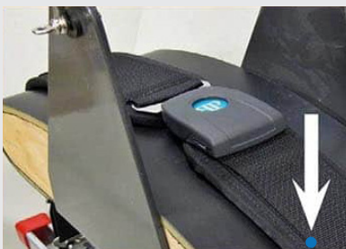
Figure 1. The blue dots on the top and bottom webbing indicate the starting position before the repetitive load is applied.
