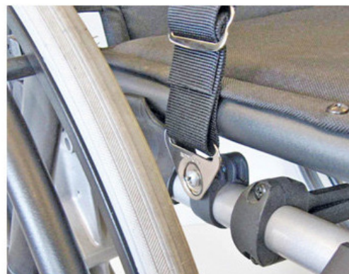
Figure 4. Triangular end-fitting and three bar slide webbing adjustment
