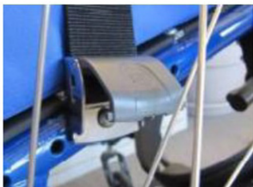
Figure 6. Locking clamp end-fitting webbing adjustment
