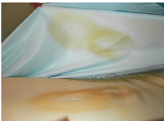
Figure 3. An example of strikethrough contamination of a foam mattress
