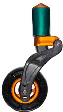
Figure 10. The Korea Institute of Machinery and Materials 'morphing' wheel
