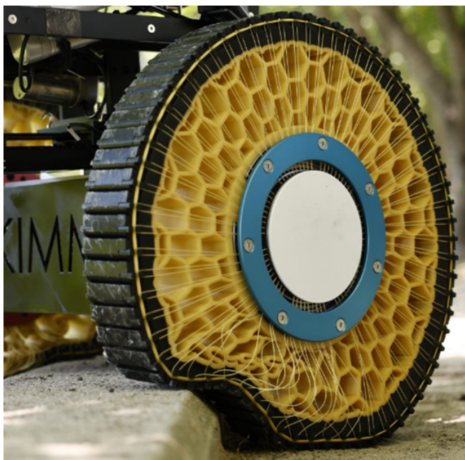
Figure 10. The Korea Institute of Machinery and Materials 'morphing' wheel
